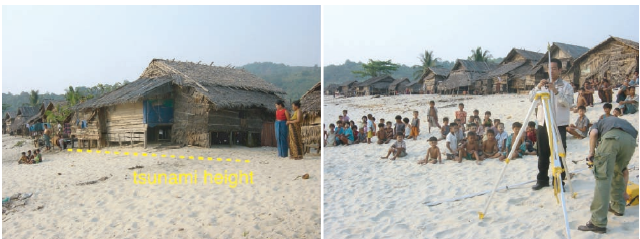
Photo 5. Survey at Sann Lan Village. Yellow dotted line is tsunami height (left). Measurement at Sann Lan Village (right).
