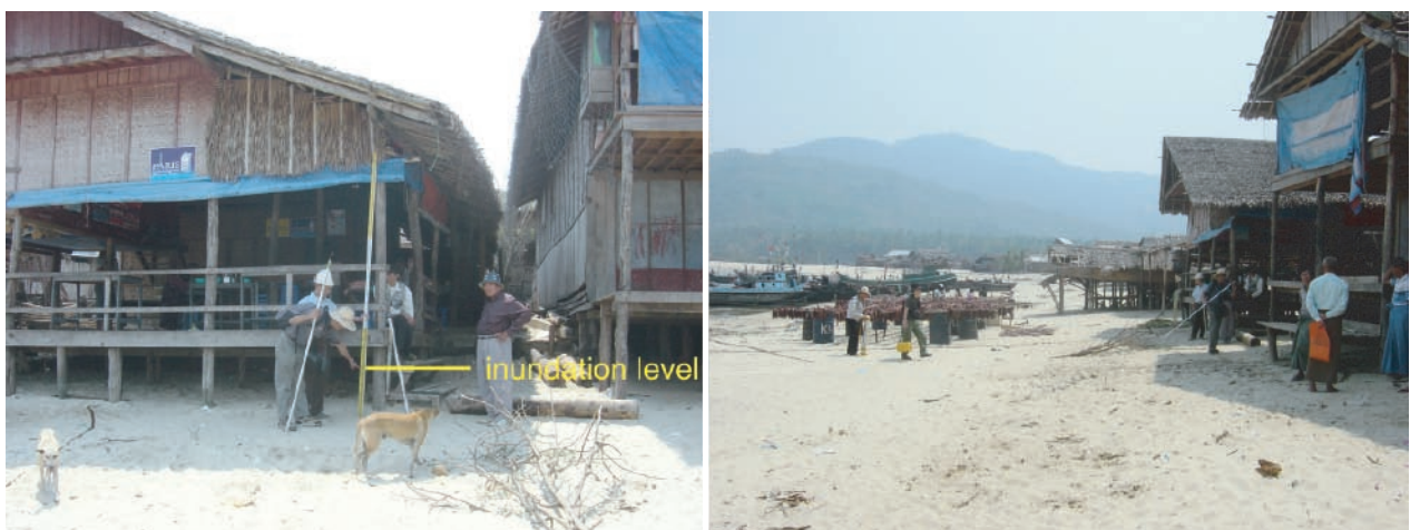
Photo 3. Survey measurement at Thabawseik-Kyauksent Village. Arrow indicates the height of tsunami (pointed by interviewee).
