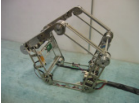
Figure 2: Our self-reconfigurable robot forming a 5R closed kinematic chain
