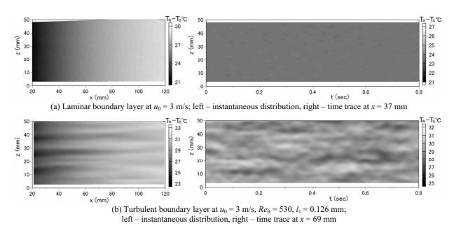
Fig. 4 Temperature distribution  $T_w - T_0$  on the titanium foil measured using infrared thermography.
