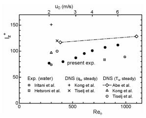
Fig. 10 Mean spacing of thermal streaks
