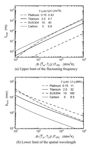
Fig. 1 Limits of the fluctuating frequency and the spatial wavelength detectable using infrared measurements.
