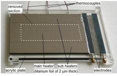
(c) Photograph of the acrylic plate Fig. 2 Test plate used in this study.
