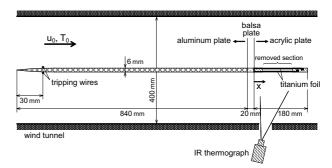
(a) Cross-sectional view of the wind tunnel
