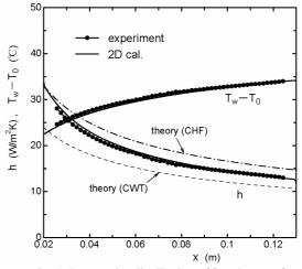
Fig. 3 Streamwise distribution of *h* and  $T_w - T_0$  for laminar boundary layer at  $u_0 = 4$  m/s.
