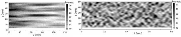
(b)  $u_0 = 3 \text{ m/s}$ ,  $Re_0 = 530$ ,  $l_\tau = 0.126 \text{ mm}$ ; left – instantaneous distribution, right – time trace at x = 69 mm
