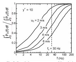
Fig. 7 Cumulative power spectrum of the velocity fluctuation in the turbulent boundary layer at  $y^+ = 10$ .
