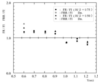
Fig. 10 Ratio of sway force of  $F_R$  and  $F_{RR}$  to  $F_I$ .
