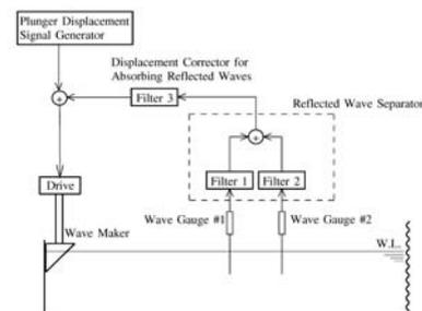
Fig. 1 Principle of absorbing wavemaker.
