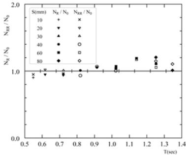
Fig. 8 Ratio of sway damping coefficients in reflecting and re-reflecting waves.
