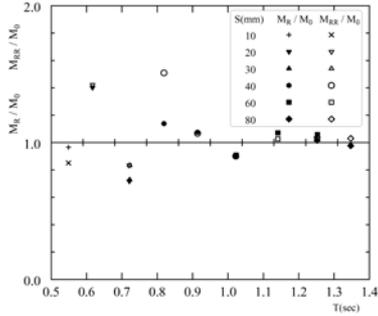
Fig. 7 Ratio of sway added mass coefficients in reflecting and re-reflecting waves.
