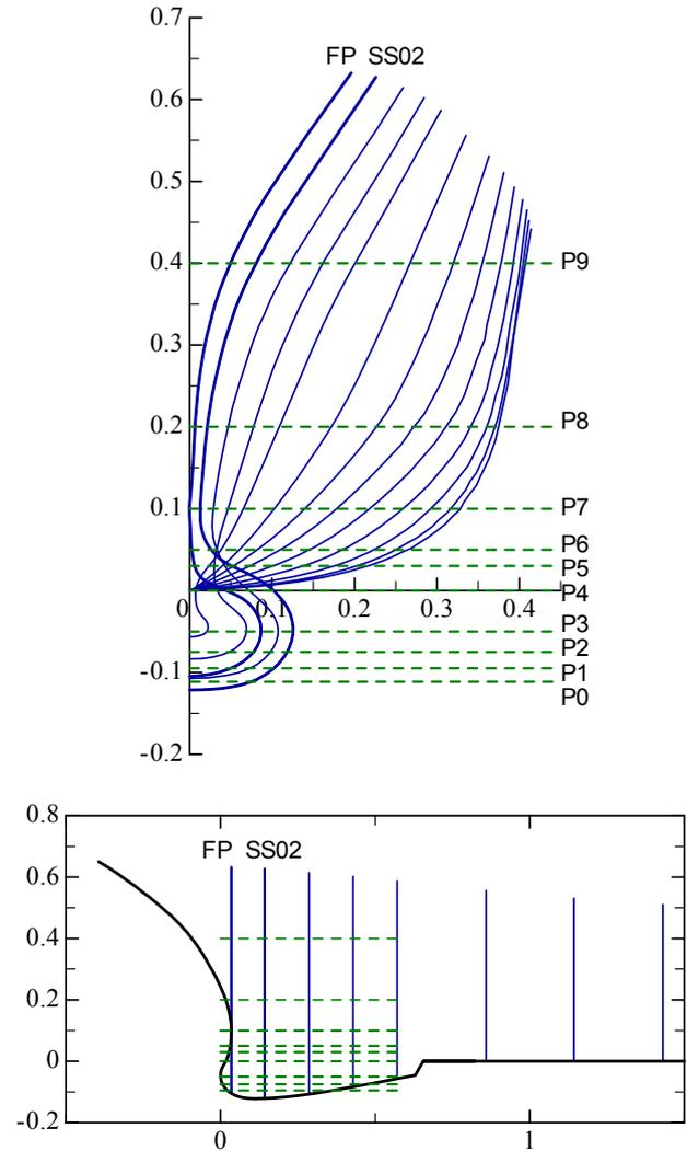
Fig.9 Body plan and profile of the Model 5415
