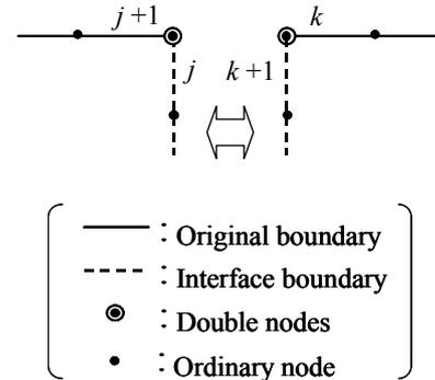
Fig.4 Node arrangement for matching domain
