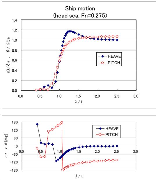
Fig.10 Computed ship motion of Model 5415
