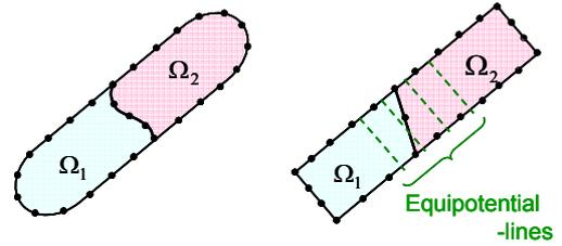
(a) Rational D.D. using BEM (b) Practical D.D. based on shallow water approximation
