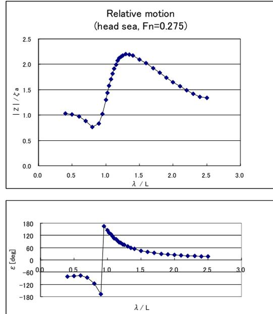
Fig.11 Computed relative motion of Model 5415
