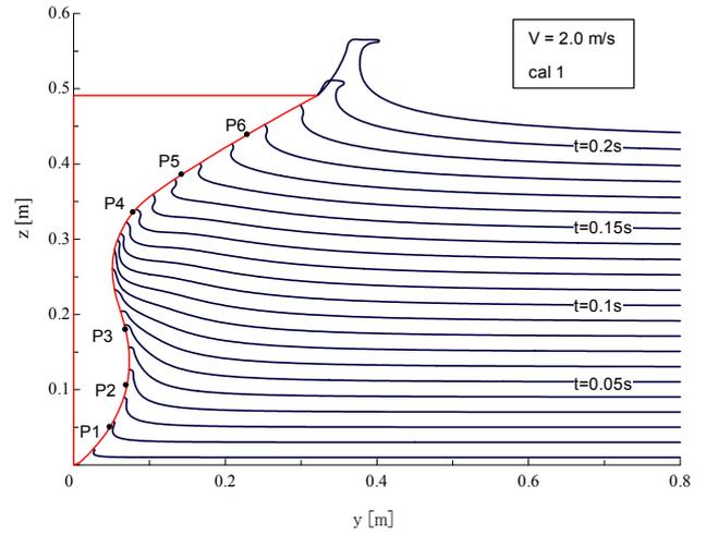
Fig.6 Computed free surface evolution in water entry
