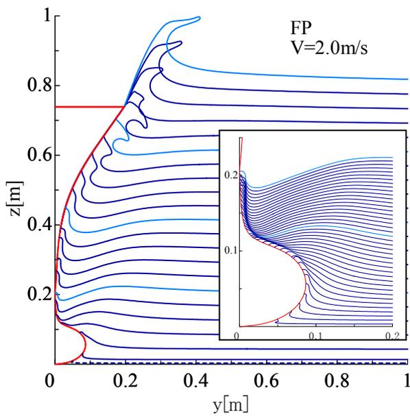
Fig.12 Computed free surface evolution in water entry
