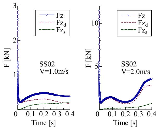
Fig.15 Vertical force on a bow section SS02
