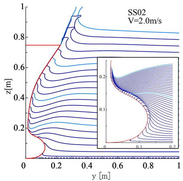
Fig.13 Computed free surface evolution in water entry
