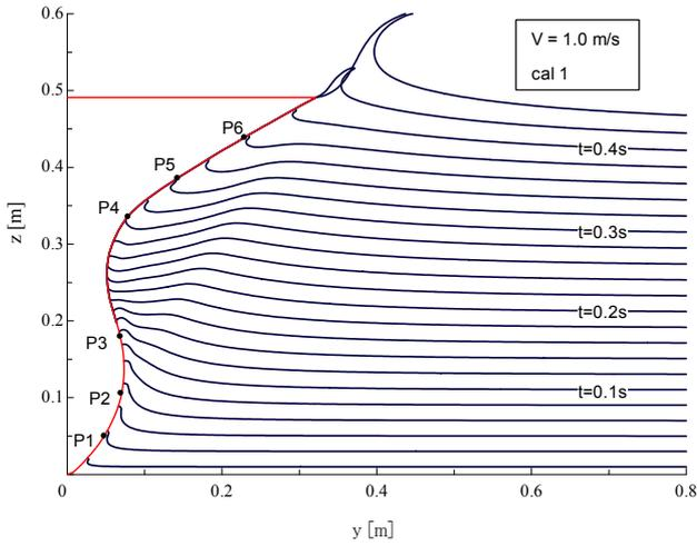
Fig.5 Computed free surface evolution in water entry
