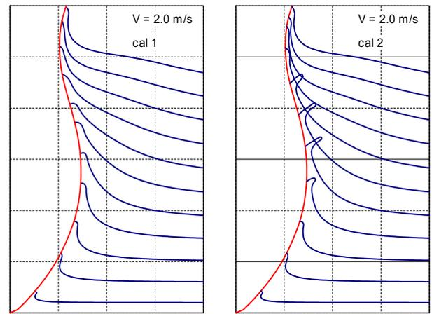
Fig.7 Comparison of computational approaches in dealing with flow detachment
