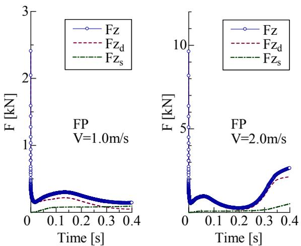
Fig.14 Vertical force on a bow section FP
