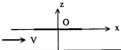
$$gh\varphi_{xx}(x) e^{i\omega_e t} + \left( \frac{\partial}{\partial t} + V \frac{\partial}{\partial x} \right)^2 \varphi(x) e^{i\omega_e t} = 0$$
